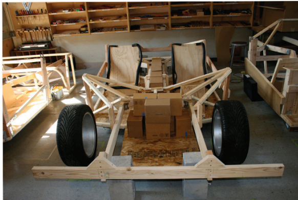
Figure 2: A wooden prototype of the X-1 Car, pre specification model
